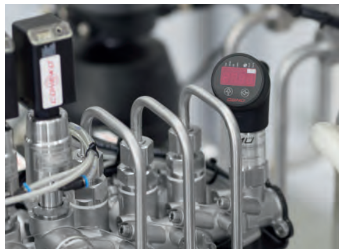
Pressure and temperature sensors
