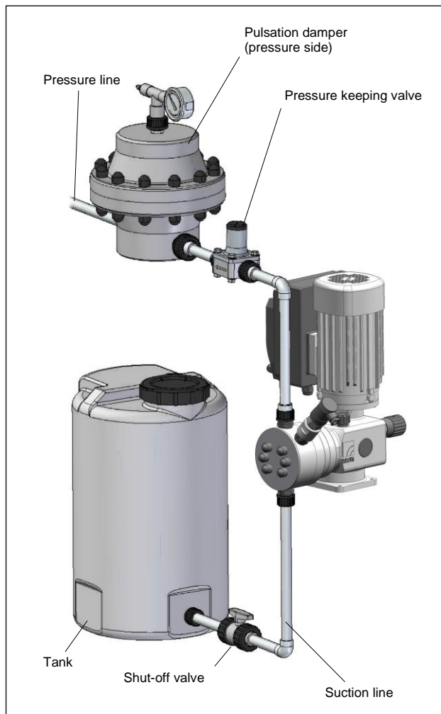
Fig. 33 Installing a pulsation damper and a pressure keeping valve
