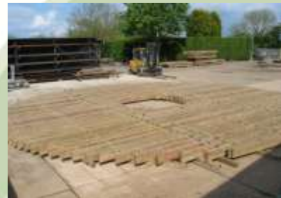
Factory check of pre-assembled timber matrix modules ready for loading onto delivery transport to site of new filter shell
