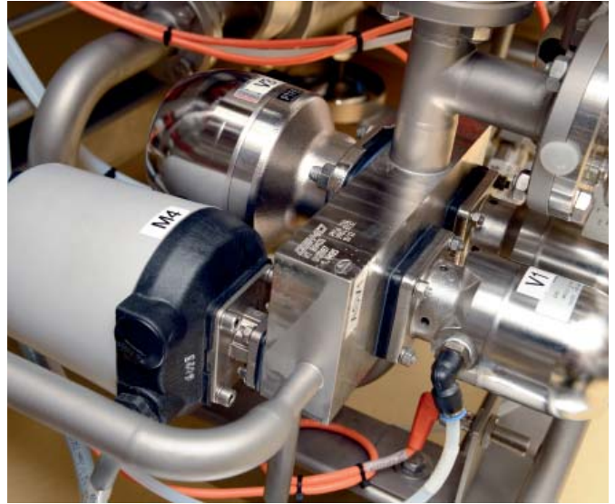
GEMÜ multi-port valve block made of stainless steel
