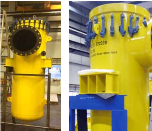
Above: VWS for SBM FPSO Ilhabellha, Mariqua and Saquerema. Total 3 x 3 Simplex Coarse Filters
