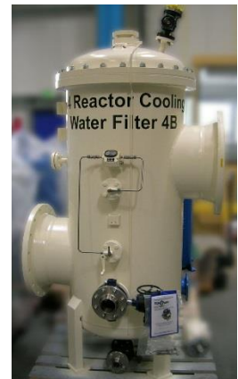
TOP & CENTRE. Hinkley Point B Power Station. Pics courtesy of British Nuclear Group. ABOVE. One of Hinkley Point's BOLLFILTERs prior to despatch.
