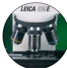
Phase contrast optics enhance views of transparent specimens
