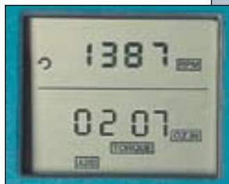
View current running speed and power, torque, flow, time, or temperature readings in the RUN mode.
