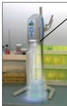
Sample light shows how well the solution is being stirred.
