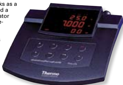
Orion 370 (58820-20) pH meter with ISE capabilities
