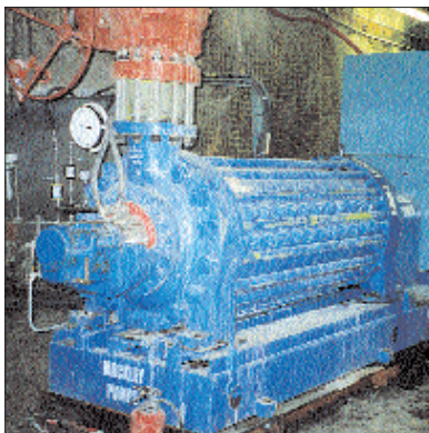
This dewatering multi-stage pump operates in Europe's deepest mine
