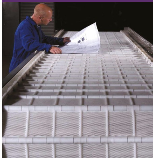
Band Screens under construction
