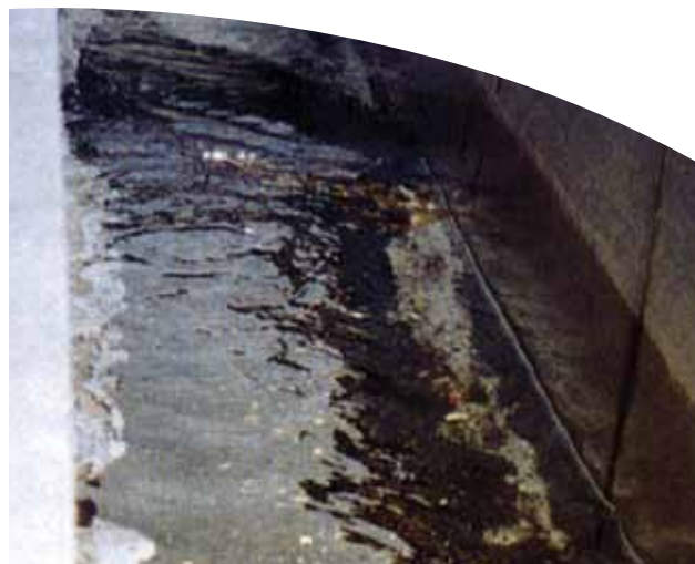
Grit undergoes washing in the constant velocity, Bache Trough.
